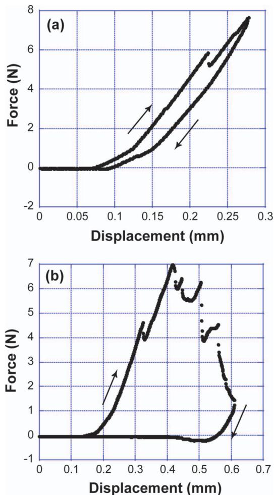
Figure 3. Representative barnacle force curves for both (a) 'hard' barnacle with 0% gummy cement and (b) a 'gummy' barnacle (90% gummy cement). Both enter linear regimes before fracture. The 'gummy' barnacles often exhibited adhesion as the punch was withdrawn.
