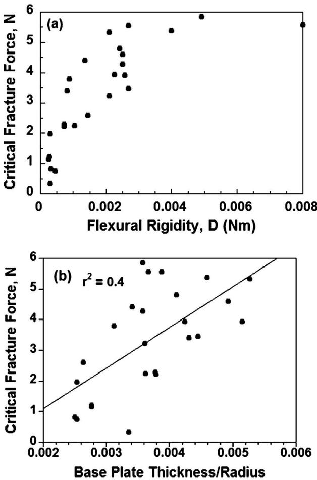
Figure 7. (a) Force required to fracture a hydrated barnacle base plate (N) plotted against its flexural rigidity (Nm) and (b) base plate thickness/radius ratio,  $t/a$ , (one-way ANOVA:  $p < 0.001$ ).
