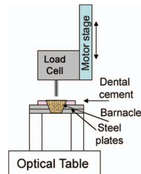
Figure 1. Punch experimental setup.
