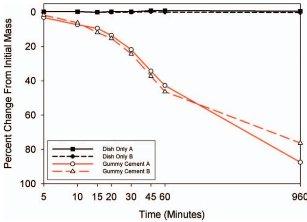
Figure 5. Gummy barnacle cement mass change over time, in air at room temperature and humidity. The cement layer was removed with a scalpel and placed in clean, 1 cm<sup>2</sup> aluminium dishes. Empty dishes were weighed as control.
