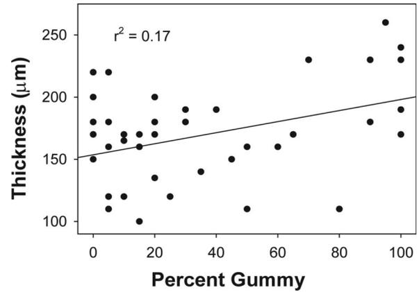
Figure 8. Thickness of the base plate ( $\mu\text{m}$ ) versus the percentage of the base plate covered in opaque, ‘gummy’ cement. This linear regression is statistically significant (one-way ANOVA:  $p = 0.006$ ).
