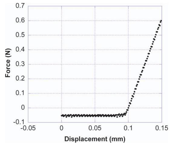
Figure 4. Portion of a force curve as the punch comes into contact with the barnacle base plate. The interaction immediately entered a linear regime, where it remained until fracture. This is consistent with the base plate being rigidly fixed in relation to the rest of the shell plates.
