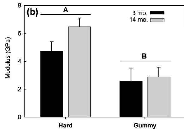
Figure 6. Flexural rigidity and modulus for (a) 3- and (b) 14-month-old gummy and hard barnacles. ‘Gummy’ is defined as >30% of the base plate covered in compliant, opaque cement, whereas ‘hard’ is defined as ≤30% of the base plate covered in compliant, opaque cement. Groups marked with A and B are significantly different (Holm–Sidak multiple comparisons,  $p < 0.05$ ).
