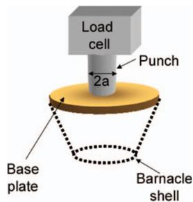
Figure 2. Detail of experimental setup, showing the physical relationship of the radius of the punch to the radius of the barnacle base plate, as described in Equations 1 and 3.
