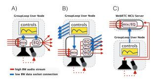
Figure 2: Potential GroupLoop networking topologies. (A) represents the current implementation, (B) shows a computationally expensive alternative, and (C) introduces a future, centralized server.
